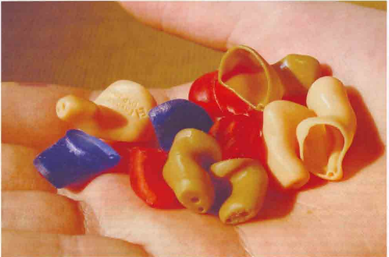
Custom-fit hearing-aid shells produced using Envisiontec Perfactory.
