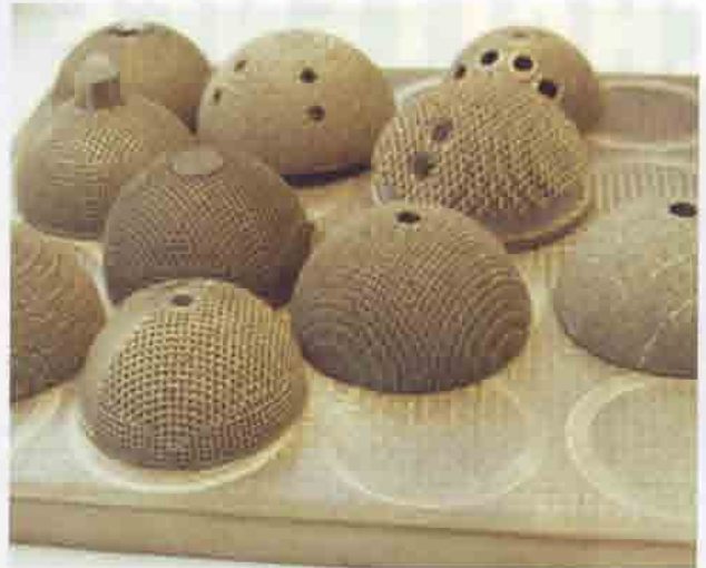
Acetabular cups manufactured using Arcam electron beam melting.
