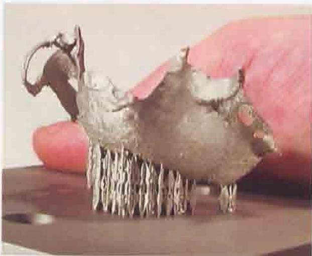
Mandible reconstruction manufactured using MCP selective laser melting.
