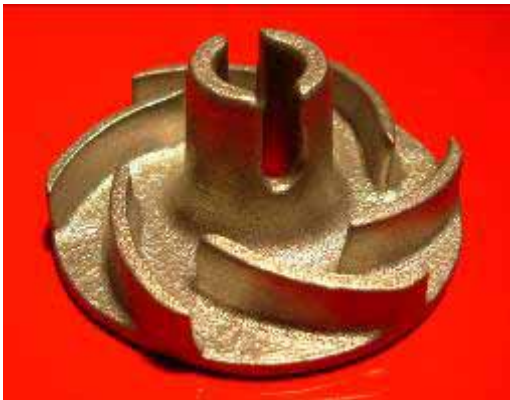
Figure 4 – Replacement classic motor cycle water pump impeller manufactured using EOS Direct Metal Laser Sintering (diameter 50mm)
