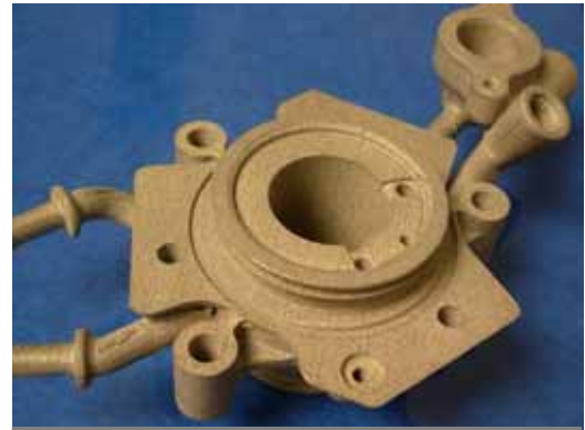
Figure 3 – Topologically optimised diesel pump housing manufactured using MCP Selective Laser Melting This part weights 60% less than the original casting
