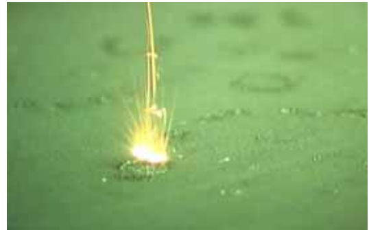
Figure 1 – Laser sintering of Cobalt Chrome powder during the build process within an MCP Realizer 100 machine
