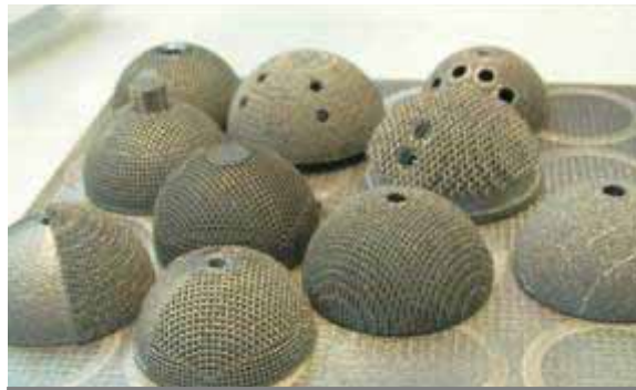
Figure 16 – Acetabular cups used as replacement hip sockets. Medical grade Titanium parts manufactured directly on an ARCAM EBM machine
