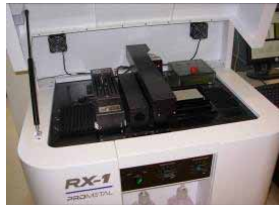
Figure 8 – Pro-Metal RX1 in-direct metal 3D Printing machine using powder and binder
