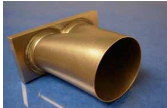
Figures 12 – Motorsport exhaust port manufactured using ACCUFUSION Laser Consolidation process (diameter 40mm)
