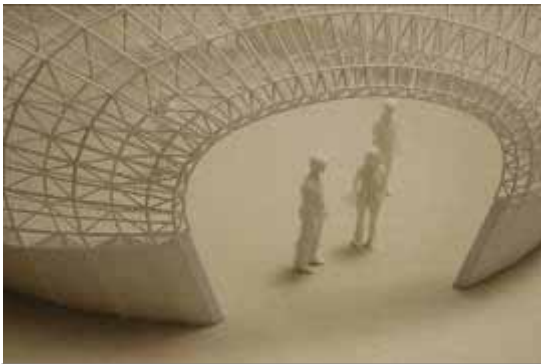
Figure 6 – Traditional polymeric rapid prototyping model manufactured using Selective Laser Sintering of Nylon
