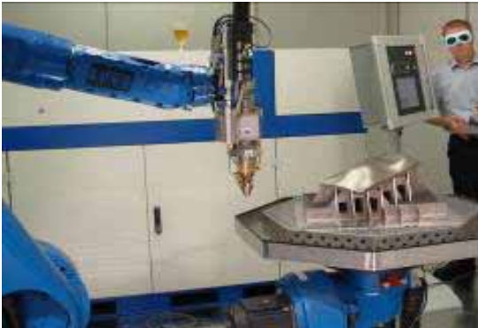
Figure 11 – Internal configuration of a TRUMPF Direct Metal Deposition Powder Feed solution using modular robot & laser
