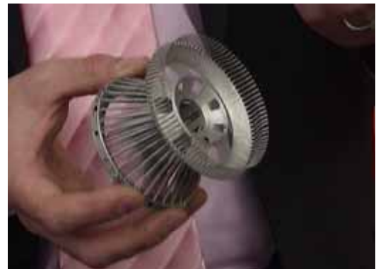
Figure 2 – Complex single piece geometry manufactured on a powder bed laser system. The part is an optical lens holder.
